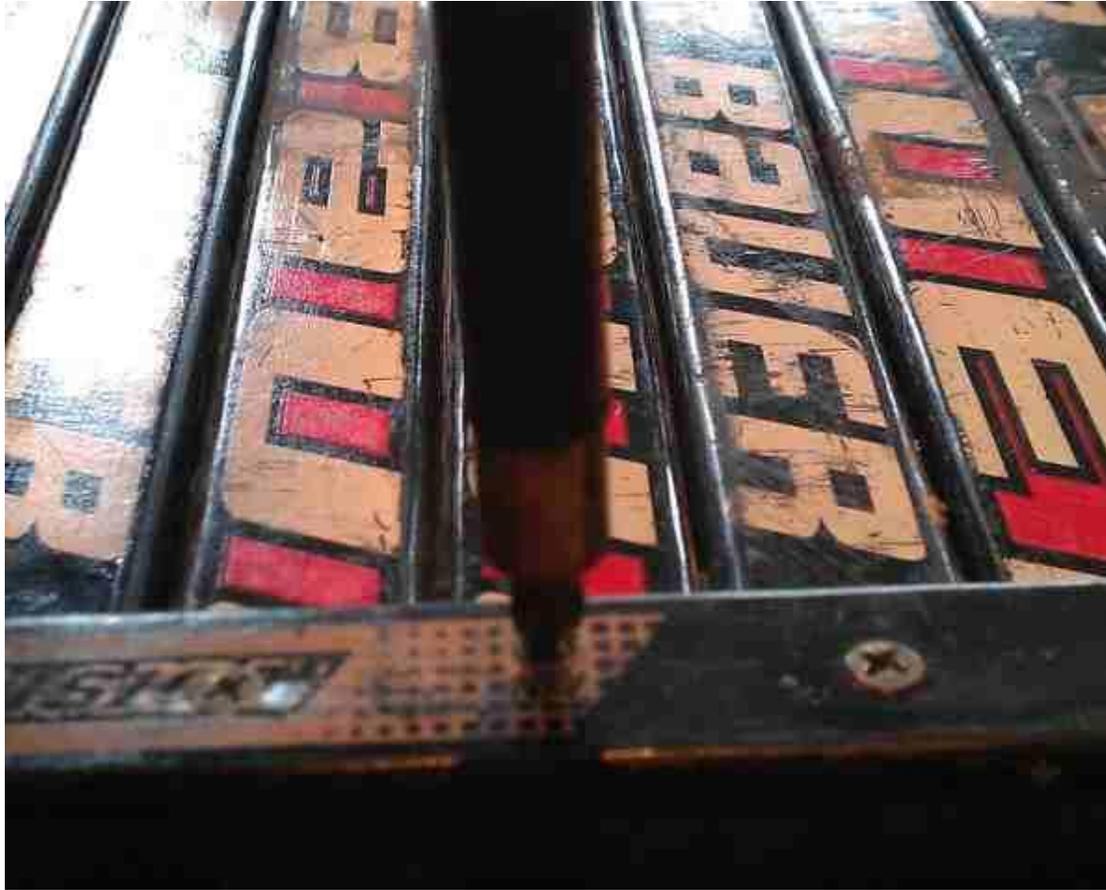
Using a circular saw and guide, cut both sides of the table. In my coffee table, the width was  $35 \frac{7}{8}$ " due to a  $\frac{1}{8}$ " loss of the blade.
